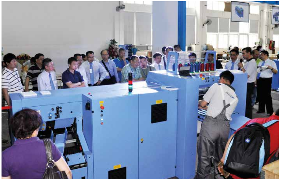
• At the open house in Shenzhen, Muller Martini demonstrated how fast the Ventura MC 160 book sewing machine and the Presto II saddle stitcher can be changed over from one job to the next.
