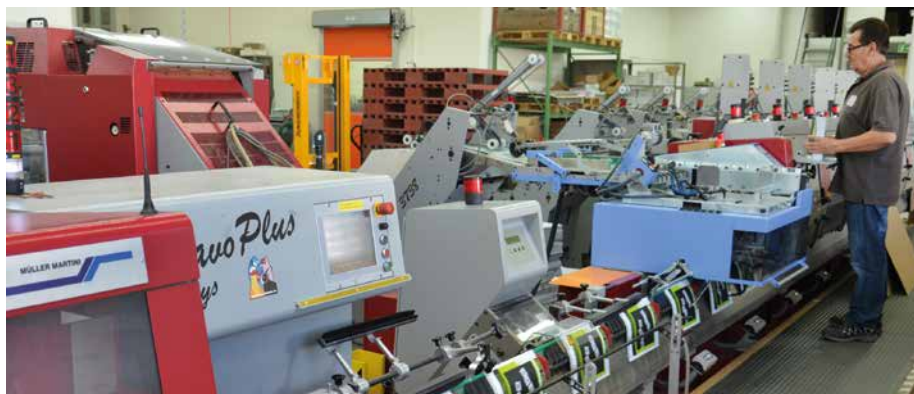
• A few months ago Zofinger Tagblatt AG retrofitted its BravoPlus saddle stitcher with the new 0507 folder feeder.
