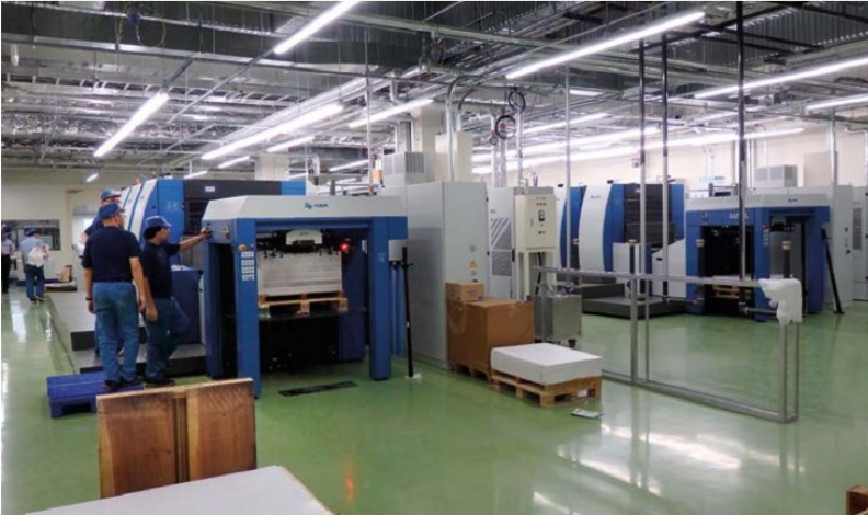
• Two Rapida 106 presses with LED-UV curing in Tosho Printing's cutting-edge press room
